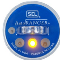
Momentary fault indication.
